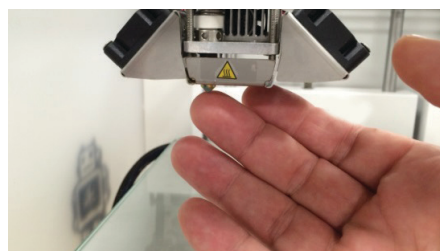
Figure III: Accessibility to heated print heads
